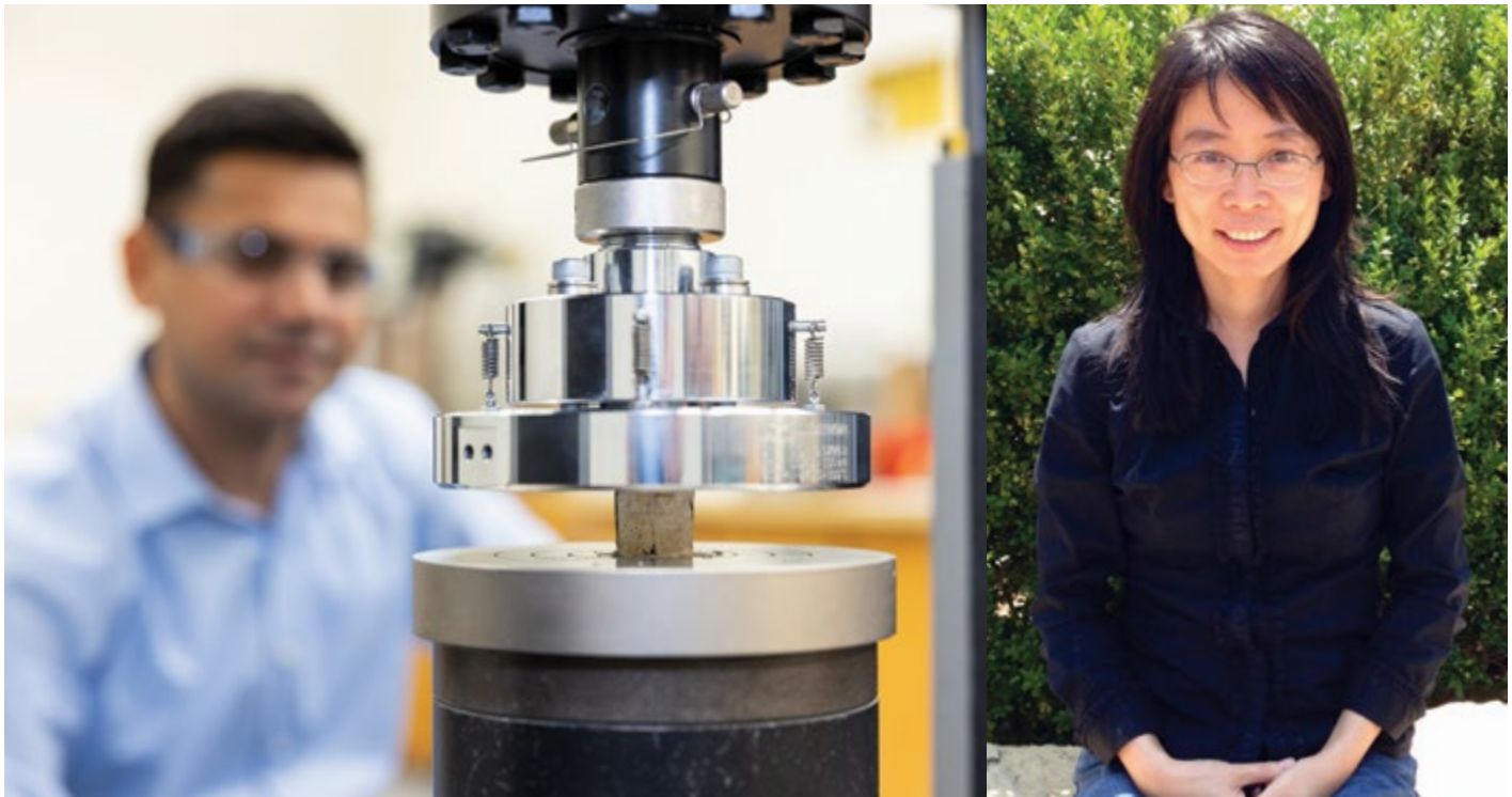
Among the many tools in Dr. Pranshoo Solanki's lab is a hydraulic press—known as a Universal Testing Machine—which he uses to test recycled roadway material to determine if it's strong enough for building roads and highways. Right , Dr. Guang Jin.
